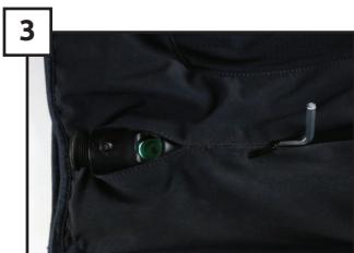
Replace the piston by using the Allen key or your finger. Make sure that the notch of the piston is in front of the hole where the key-ball is placed.
