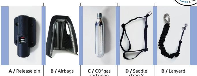
● **A Release pin.** The tractive force required to trigger the airbag varies according to the airbag's size (Child S up to XL). The ball is ejected; the spring relaxes and transmits energy to the needle that pierces the cartridge, instantly releasing the gas that inflates the airbag. For your own safety and proper functioning of the airbag system, do not dismantle the release pin or remove any parts
